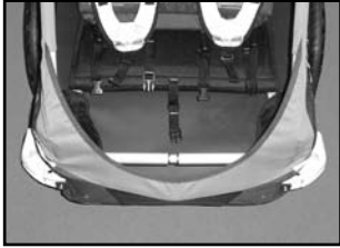
Fitted telescopic tube, shown from the front.
